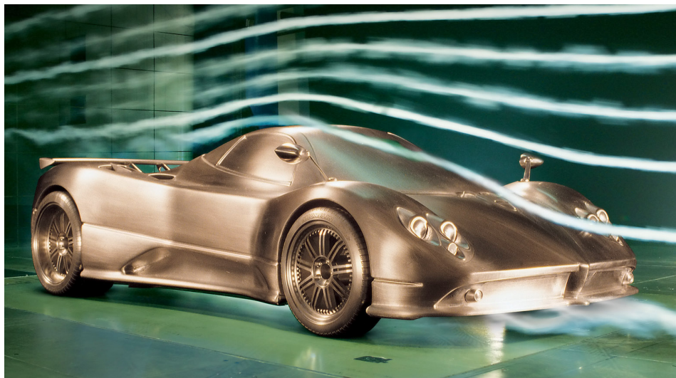
Figure 1.1: Real-world examination of a sports car prototype in a wind tunnel [Pag05]. The airstream is visualized by smoke released from several dies.
